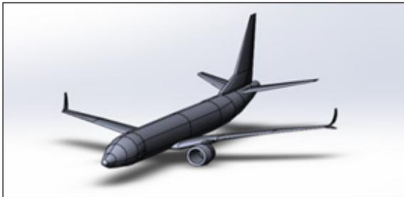
**Fig.3 - 3D-model of the Boeing-737-800 with Split-tip tips**
